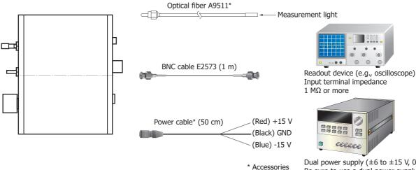
Dual power supply ( $\pm 6$  to  $\pm 15$  V, 0.1 A or more) Be sure to use a dual power supply. Switching power supplies are not supported. Use a series power supply (ripple voltage: 3 mVp-p or less).
